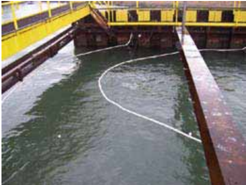
C.I. Agent® Marine Booms used for polishing sheen after out-fall at utility power plant.
